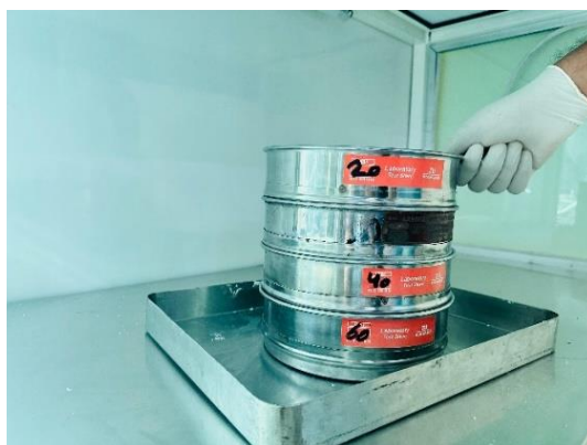
Figure 2: Sieve Stack for Particle Size
