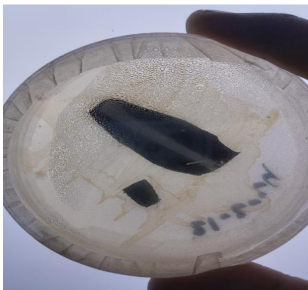
Fig 5: Polyester Fabric as Negative Control, not Coated with Any Compound
