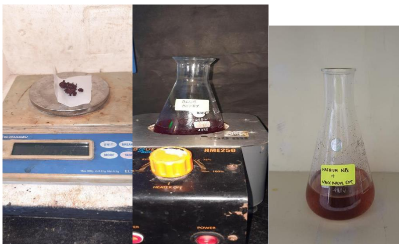
Figure: 1. Preparation of nanoparticles using Vaccinium sect. Cyanococcus plant extract Powder was weighed (b) Boiling of the Plant extract (c) Hafnium oxide nanoparticles
